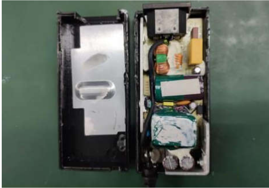
Figure 7 Components side view of all unit (Fuse:F1 and F2)
