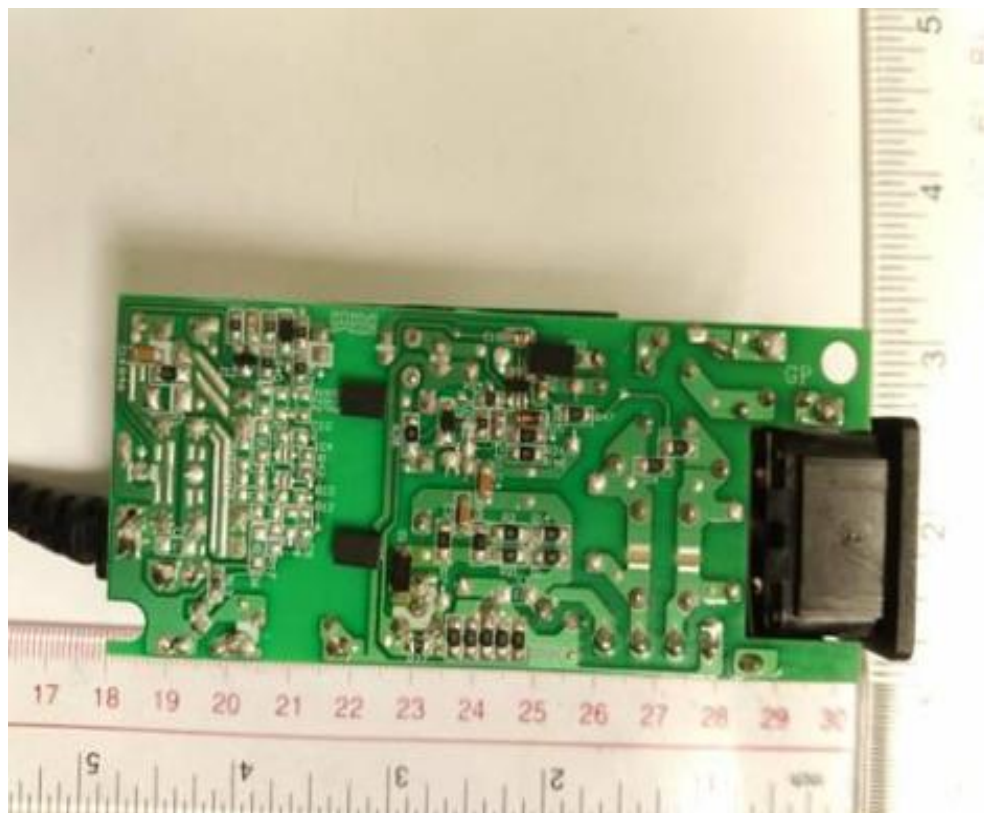
Figure 24 PCB trace side view of all unit (For 2ABF and 2ACL (with LED))
