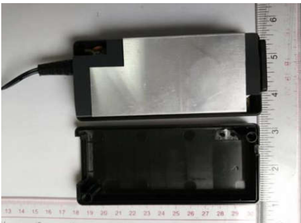
Figure 14 Internal view of unit (For 2ABF and 2ACL (with LED))
