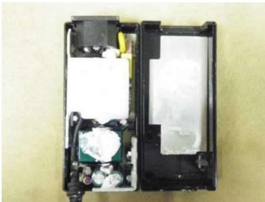
Figure 6 Internal view of unit (Fuse:F1 and F2)
