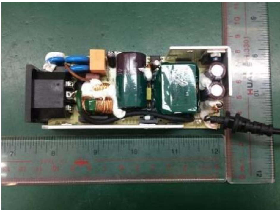
Figure 10 Components side view of all unit (Fuse:F1 and F2(with TVS2, TVS3, TVS4))
