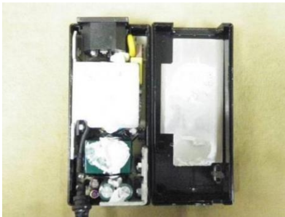
Figure 6 Internal view of unit (Fuse:F1 and F2)
