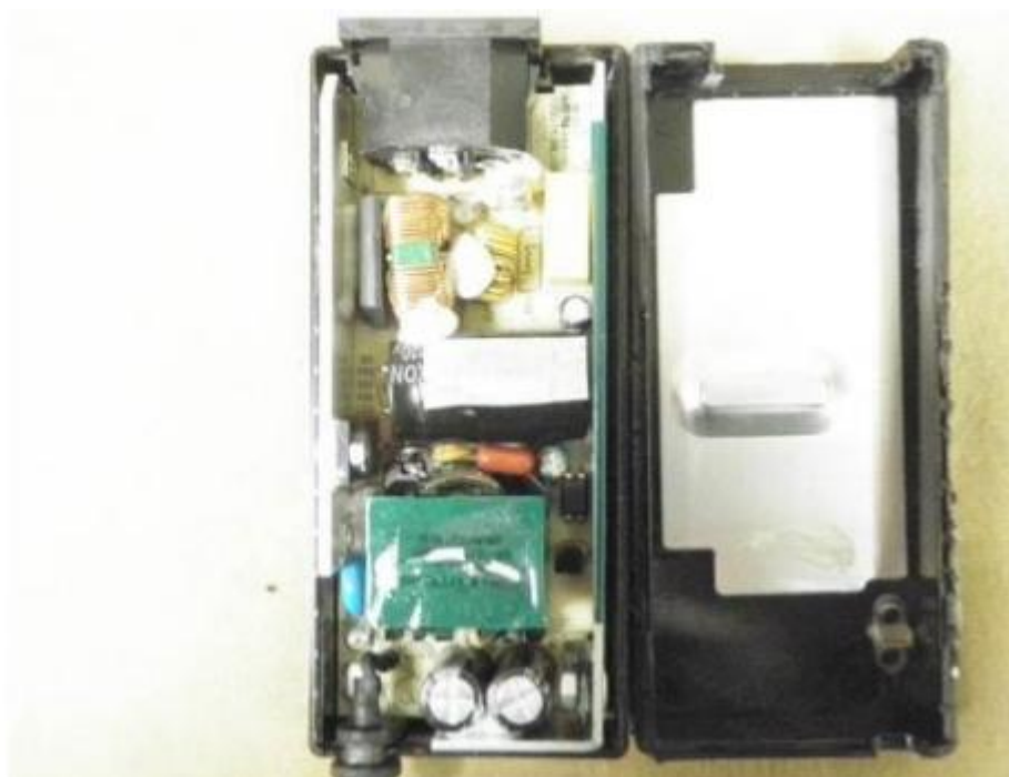
Figure 3 Internal view of unit (Fuse:F1)
