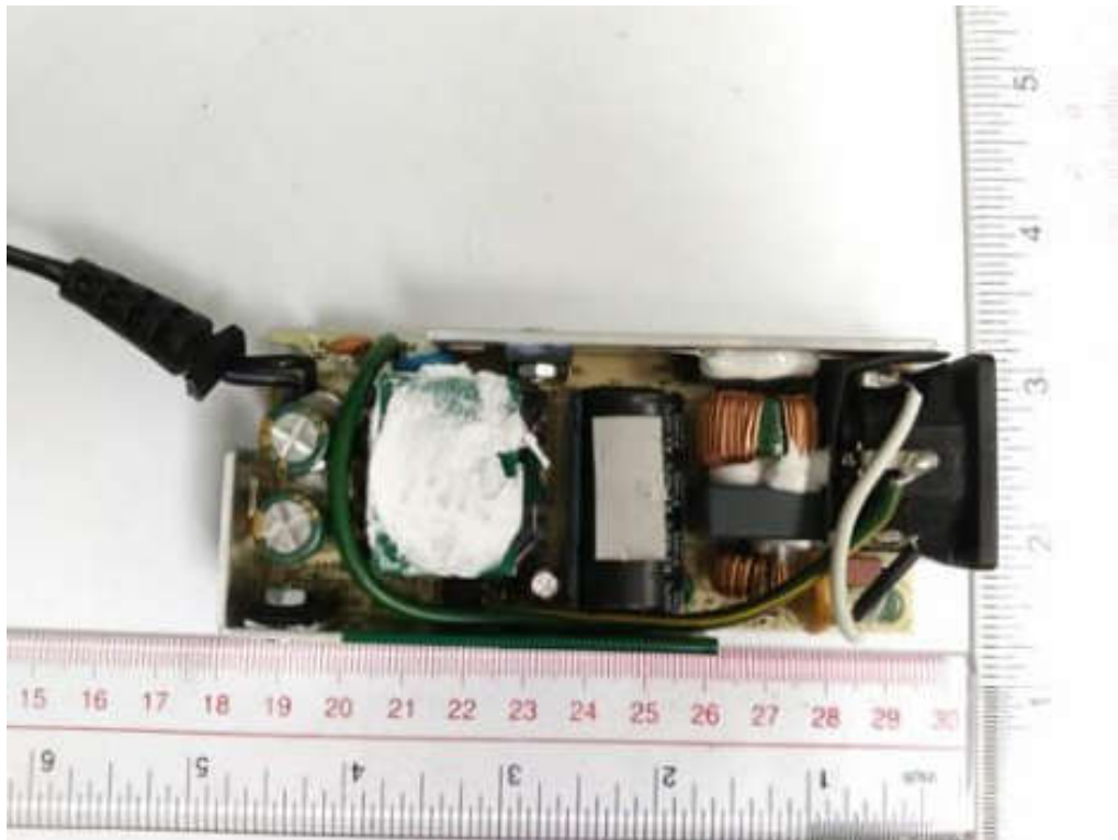
Figure 15 Components side view of all unit (For 2ABF and 2ACL (with LED))
