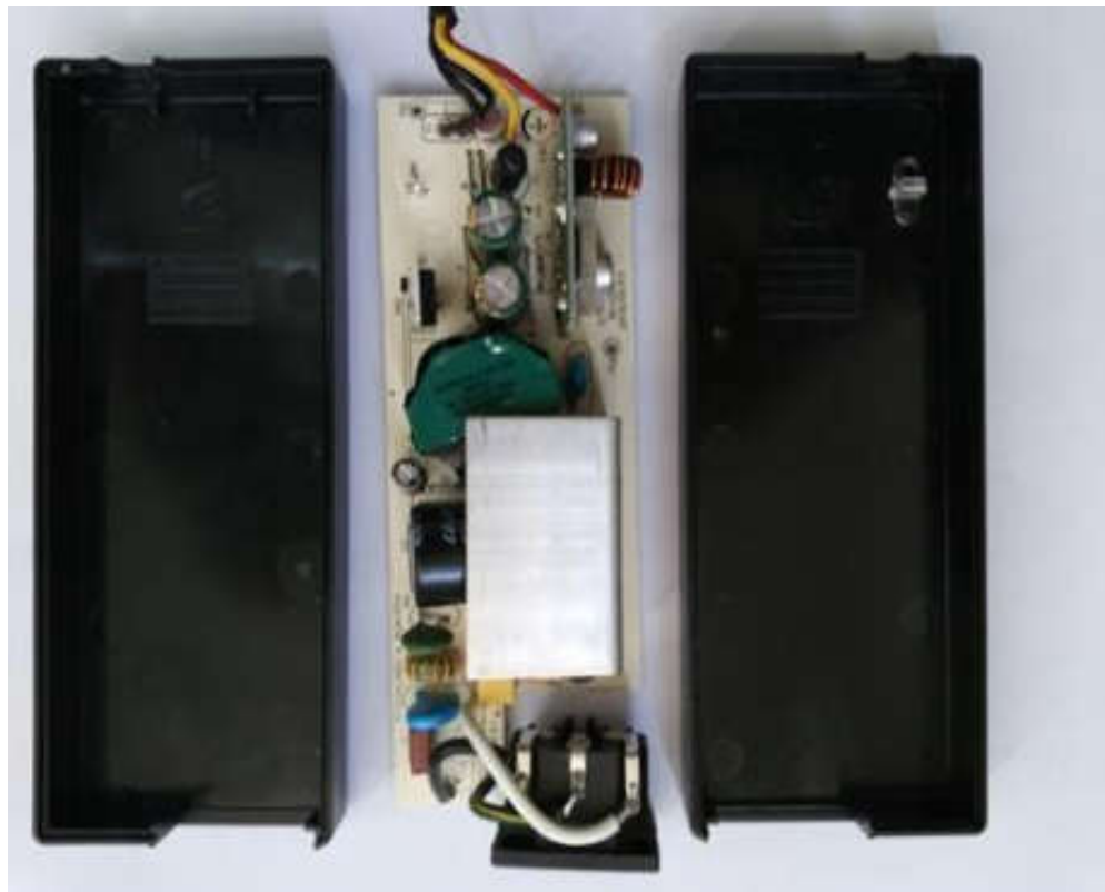
Figure 14 Internal view of unit (For GTRxxxYzzzzz)
