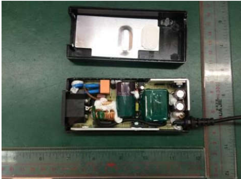
Figure 9 Internal view of unit (Fuse:F1 and F2 (with TVS2, TVS3, TVS4))
