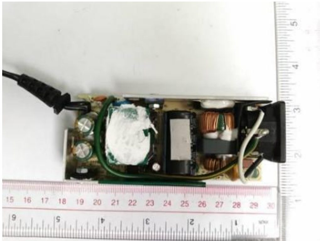
Figure 23 Components side view of all unit (For 2ABF and 2ACL (with LED))
