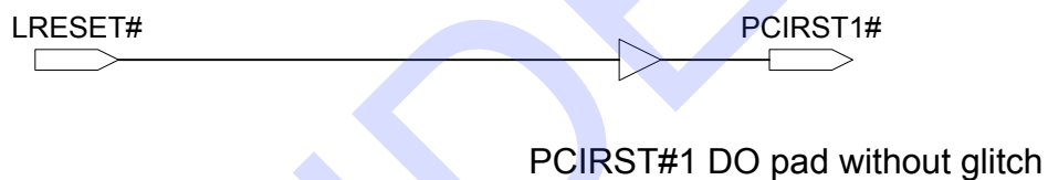
Figure 11-15. PCIRST#1 Signal Timings
